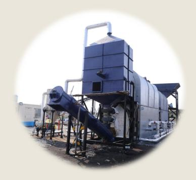
Torrefaction is a thermal treatment process that involves heating RDF/MSW/AGRO **WASTE/STP SLUDGE** materials (typically between 200°C to 350°C) in the absence of oxygen, to remove its moisture and volatile organic compounds and to increase its energy density. The result is a product known as "Eco Green Coal" which is a dry, brittle and carbon-rich product that can be used which holds a calorific value of 3500-4000 kcal/kg.
